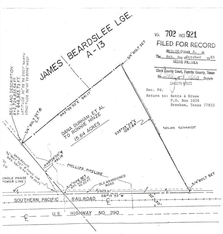
NOTE: All bearings, distances and coordinates shown hereon refer to the Texas Plane Coordinate System - South Central Zone, as determined from the Carmine Triangulation Station.
